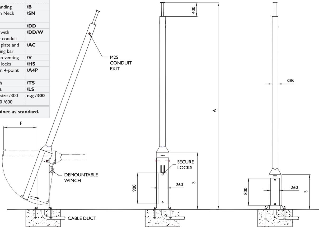
Pole is fixed in the vertical position using 2 no. bolts and locked with internal nuts - has the facility to be padlocked internally to stop unauthorised tilting.
